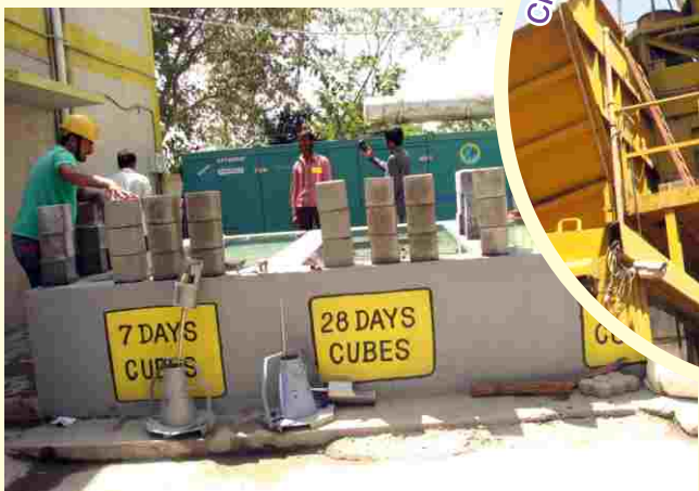
Curing Tank containing Age wise Concrete Cubes
